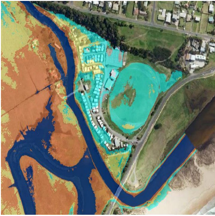
Subject property showing the 1% AEP riverine flood depth mapping coinciding with a 10% AEP storm tide event based on 2030 climatic conditions on the left, and 2100 climatic conditions on the right
