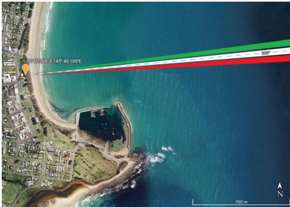
Figure 4 Foreshore Sector Light
